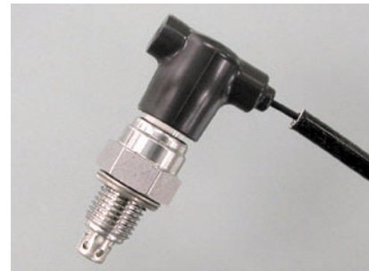
Fig. 1 External view of developed heaterless O 2 sensor
