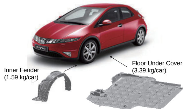
Fig. 4 Floor Under Cover and Inner Fender for 06 model year CIVIC
