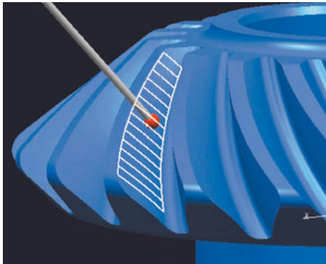
Fig. 8 Nominal data line generated on reverse actual model
