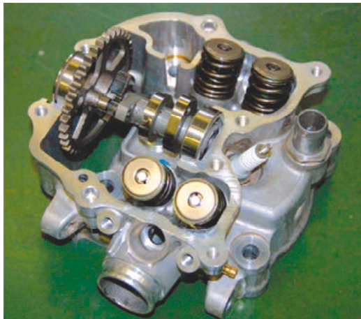
Fig. 13 Cylinder head with valve system
