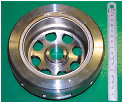
Fig. 8 AC generator flywheel
