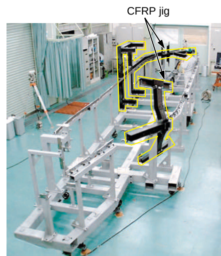
Fig. 8 CFRP/steel assembly jig
