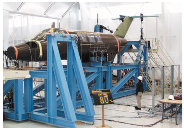
Fig. 17 Fuselage proof test
