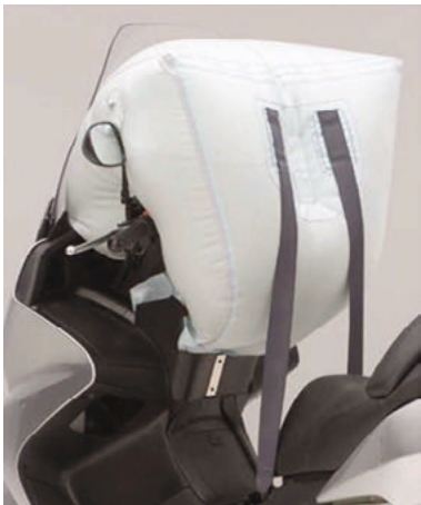
Fig. 6 Prototype airbag system for large scooter
