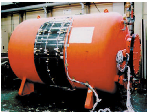
Fig. 14 Sub-component test of passenger door
