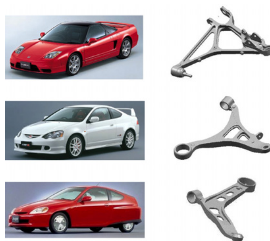
Fig. 1 Applied examples of forged aluminum suspension arms
