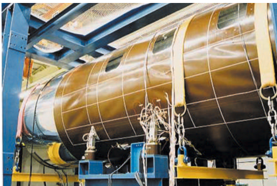
Fig. 16 Skin buckling at limit load
