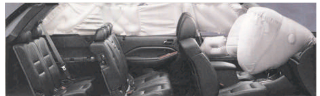
Fig. 5 Deployed front airbags, side airbag and side curtain airbag
