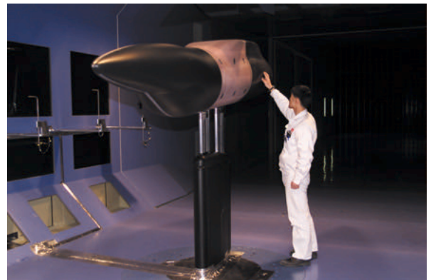
Fig. 9 1/3-scale fuselage model for NLF nose test
