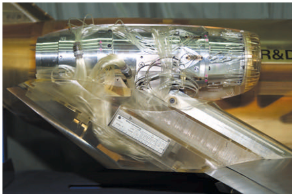
Fig. 7 1/6-scale engine simulator
