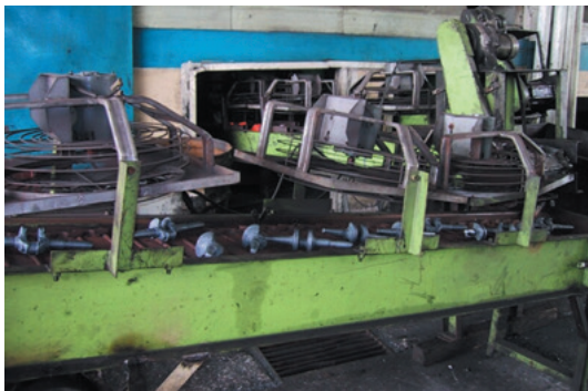
Fig. 2 Fan cooling after hot forging
