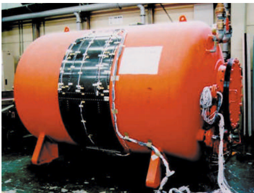
Fig. 14 Sub-component test of passenger door
