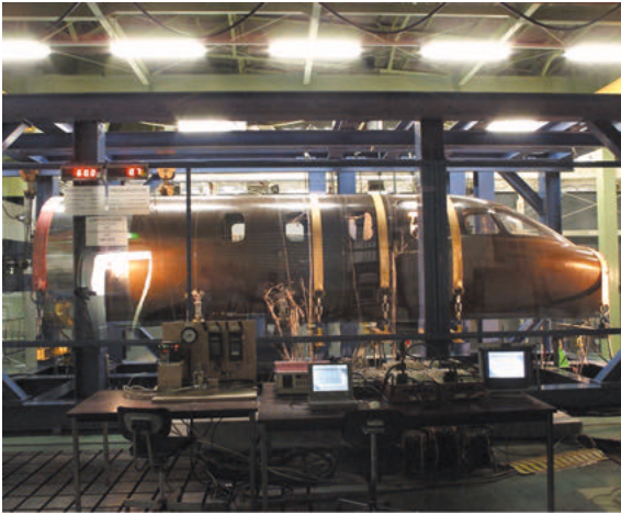
Fig. 15 Cabin component test
