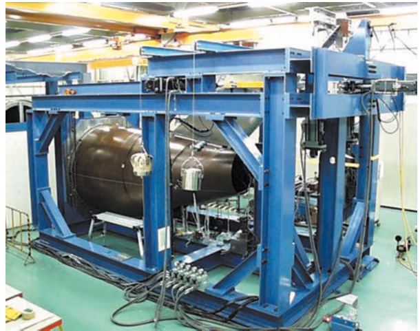
Fig. 18 Tail component test
