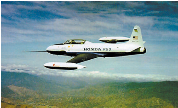
Fig. 4 T-33 aircraft modified for NLF flight test
