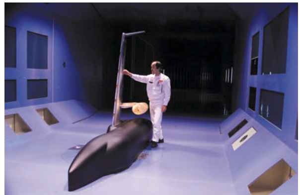
Fig. 6 1/3-scale low-speed wind tunnel model
