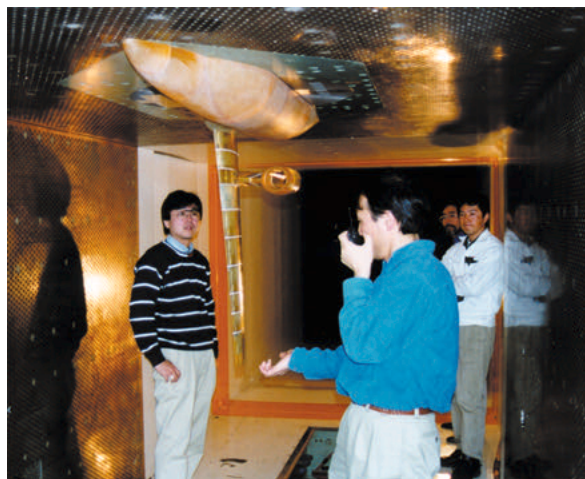
Fig. 13 Transonic wind tunnel flutter test at JAXA transonic wind tunnel
