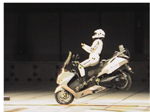
Fig. 2 Motorcycle and dummy in simulated curb ride over test
