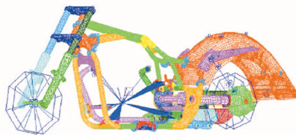
Fig. 12 Complete motorcycle FE model
