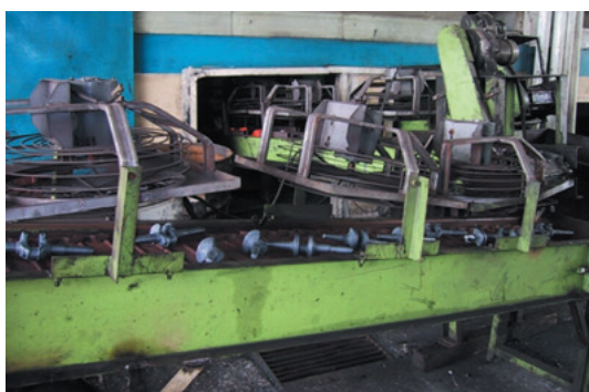
Fig. 2 Fan cooling after hot forging
