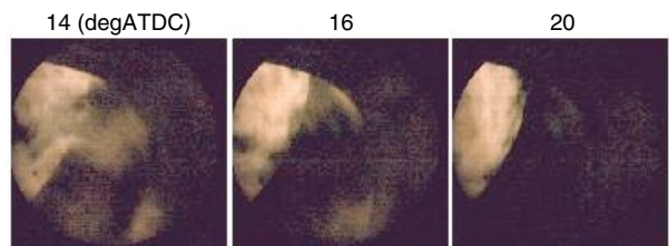
Fig. 7 Effect of nozzle cone angle on flame behavior (CCD camera)
