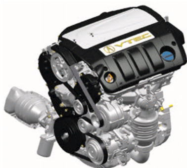
Fig. 5 View of V6 SOHC-VTEC engine
