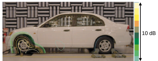
Fig. 12 Result of beamforming analysis
