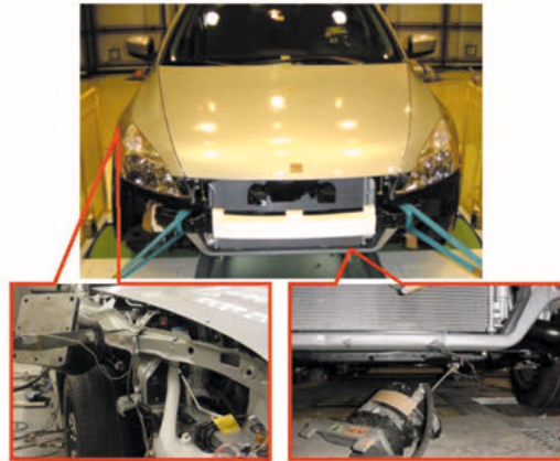
Fig. 1 Excitation points in operational EMA
