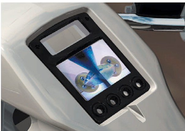
Fig. 10 Monitor of outrigger position
