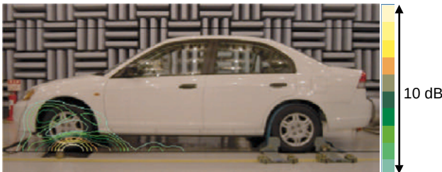
Fig. 17 Result of beamforming (without exhaust noise radiation)
