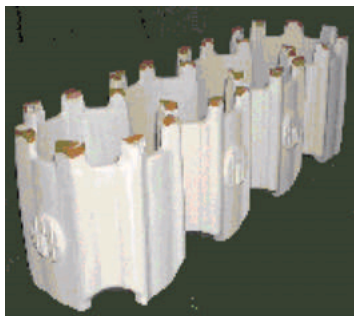
Fig. 22 External view of pressure-resistant sand cores
