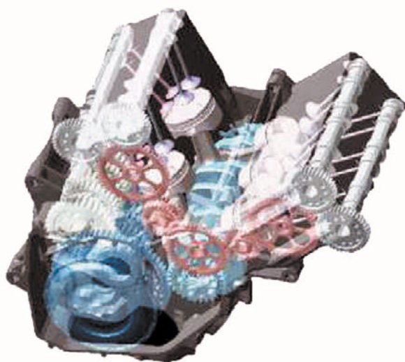
Fig. 4 Cutaway drawing of RC211V engine
