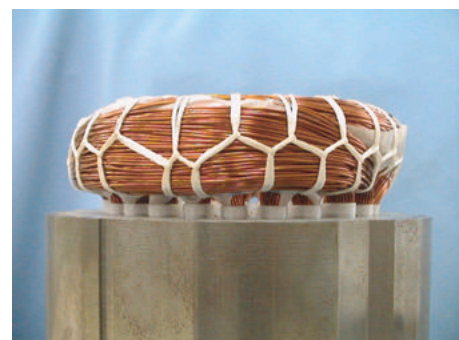
Fig. 3 Winding overhang produced by insert coil machine
