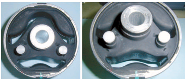
Fig. 15 Engine mount after endurance test
