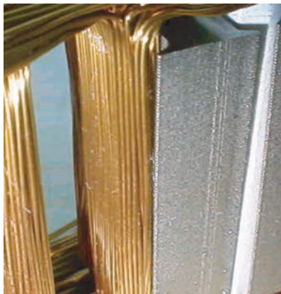
Fig. 11 Winding aligned inside a slot
