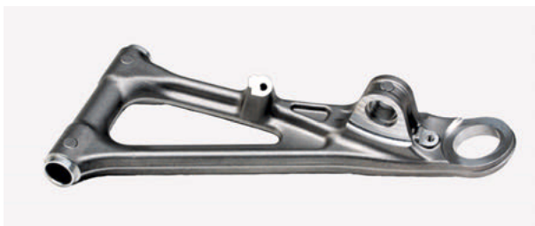
Fig. 21 Aluminum forged front upper arm
