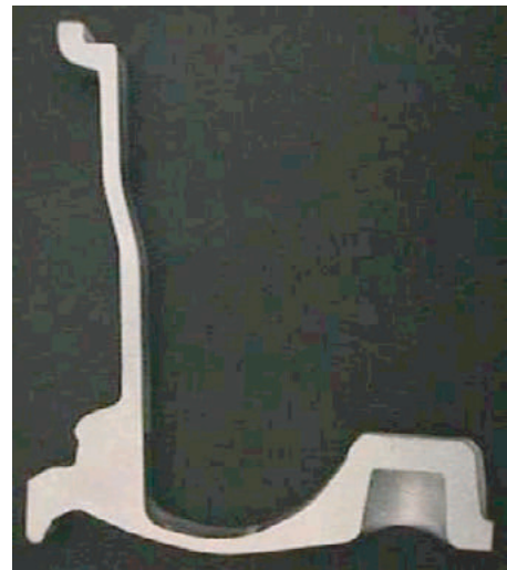
a) New multi-gate LPDC process
