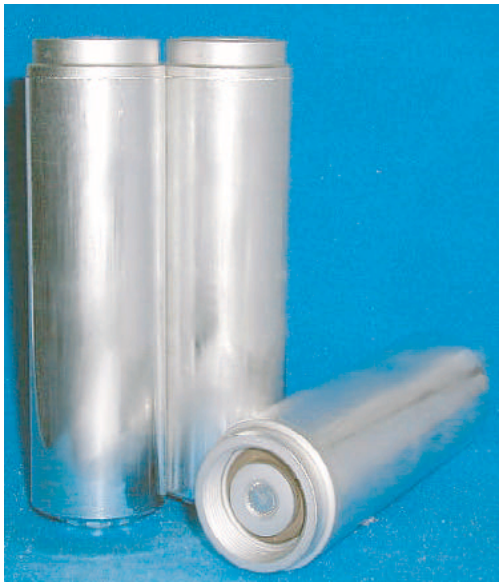
Fig. 4 Photograph and cutaway view of Honda Ultra capacitor
