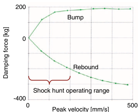
Fig. 8 Rock damper damping force
