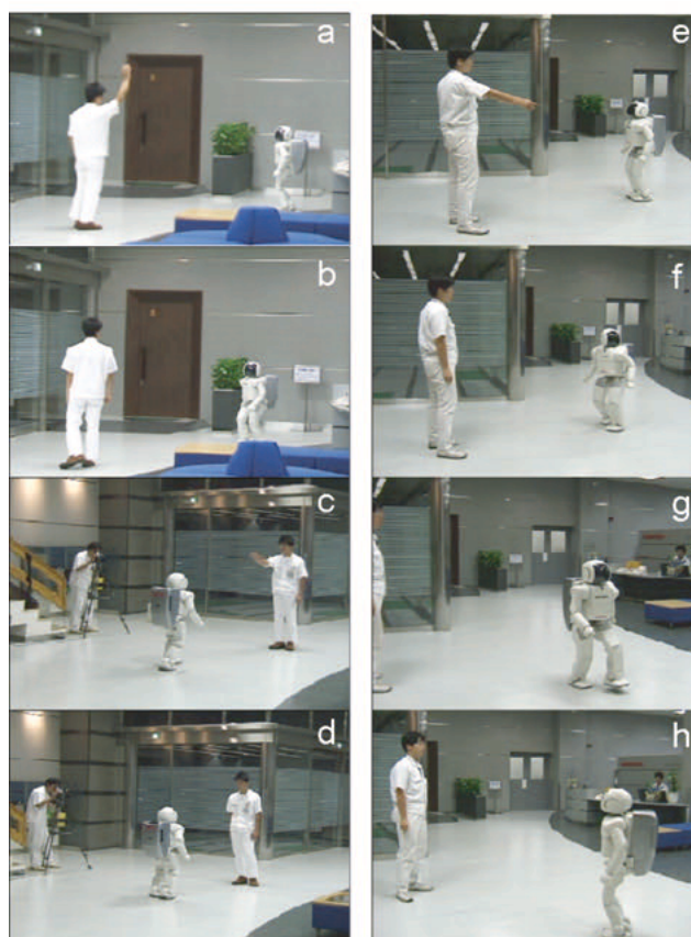
Fig. 16 Demonstration images a: recognize “high-hand” posture, b: start to follow, c: recognize “stop” posture, d: stop walking, e: recognize pointing position, f: start to walk, g: walk to pointing position, h: arrive and stand by
