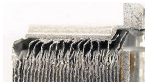
Fig. 6 Detail of welded area on electrical contact points
