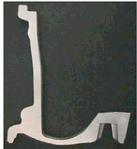
b) Side-gate LPDC process
