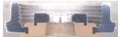
Fig. 10 Cut section of cover
