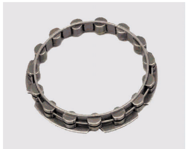
Fig. 9 External view of one-way clutch
