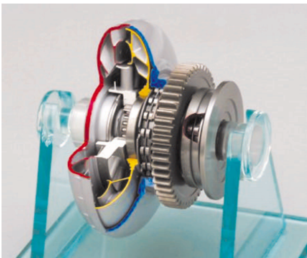
Fig. 5 Cutaway model of torque converter
