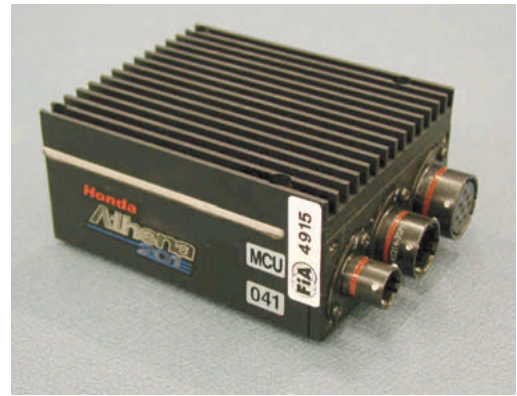
Fig. 7 Motor control unit (MCU)
