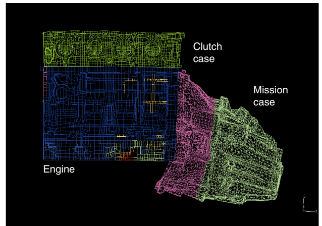
Fig. 18 FEM simulation of resonance frequency analysis at bending mode in the vertical direction
