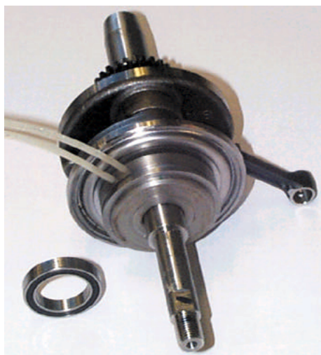
Fig. 20 Crankshaft with water cooled bearing
