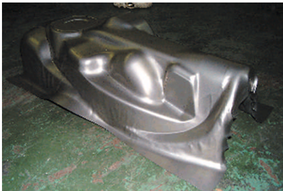
Fig. 12 Result of press forming with arbitrary die face
