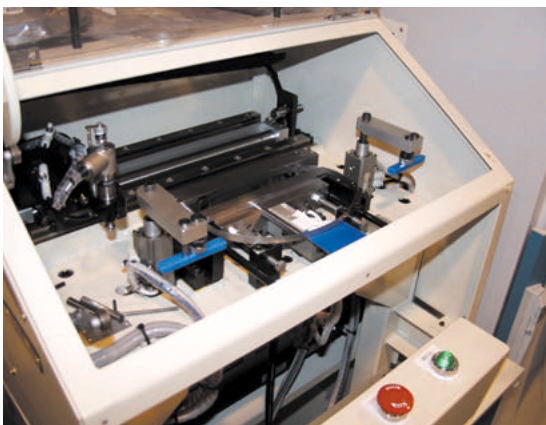
Fig. 13 Automatic machine for ring curve measuring [Made by: Honda Engineering CO.,LTD]
