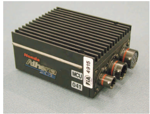
Fig. 7 Motor control unit (MCU)
