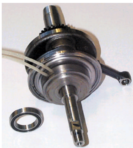
Fig. 20 Crankshaft with water cooled bearing
