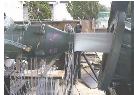
Fig. 16 Test equipment for water jet pump in operating
