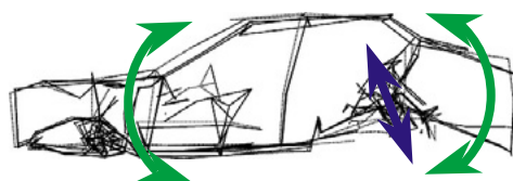
Fig. 7 Body 2nd bending shape (実挙動解析)
