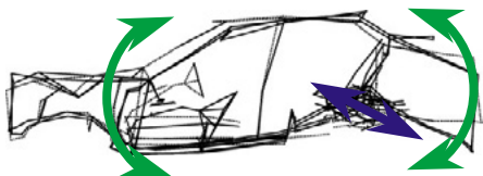
Fig. 5 Body 2nd bending modal shape (台上モーダル解析)
