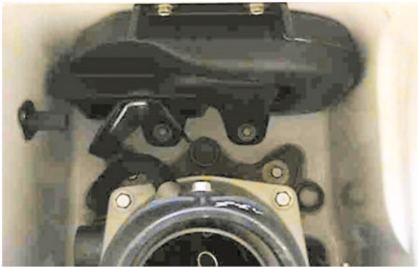
Fig. 20 Installed appearance of water chamber (Resonator)
