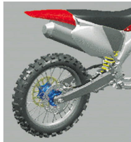
Fig. 25 Structure of rear suspension
