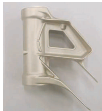
Fig. 24 Forging aluminum steering head pipe
