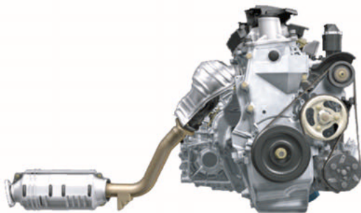
Fig. 22 View of exhaust system
