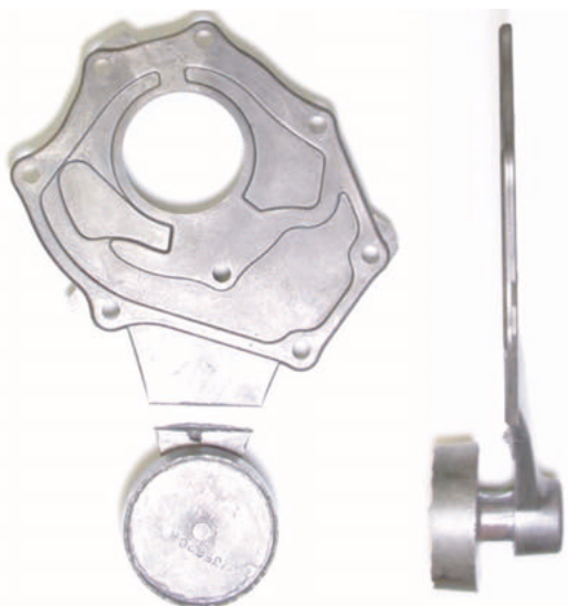
Fig. 15 As-cast oil pump cover
