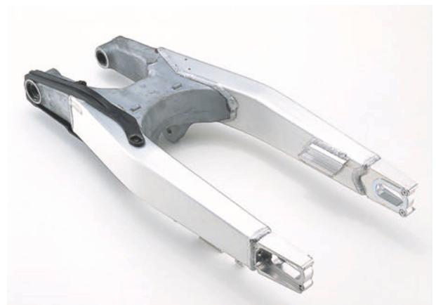
Fig. 26 External view of swing arm
