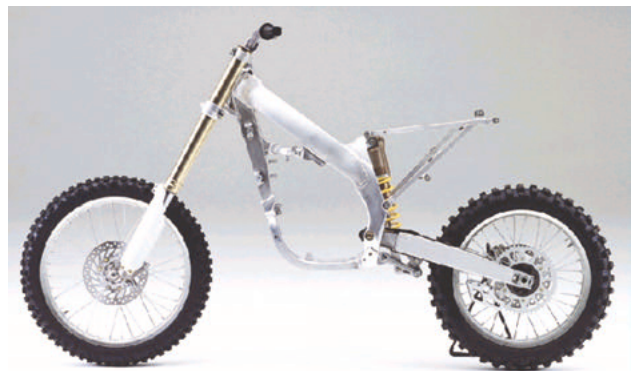
Fig. 23 External view of frame
