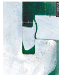
Fig. 4 Section of pulley crack
