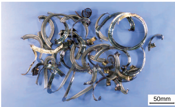
Fig. 2 Chips of sulfur free-cutting steel generated by lathe turning
