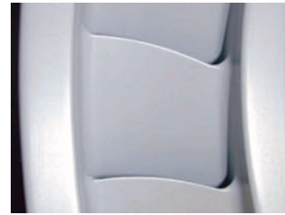
Fig. 22 Finished surface of SLA (Primer coated)
