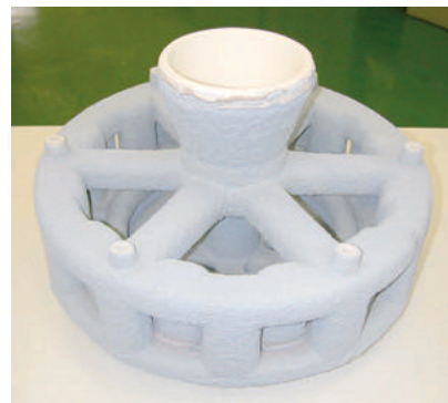
Fig. 7 Ceramic shell mold of turbine nozzle
