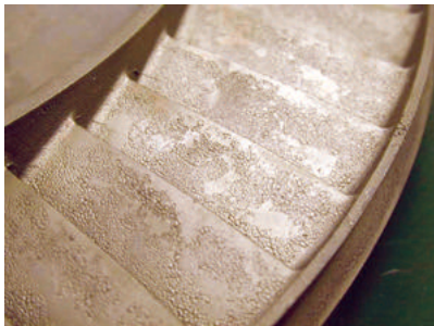
Fig. 10 Orange peel (Cast)
