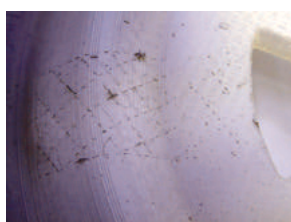
Fig. 21 Primer coated surface of SLA (Remains of support)
