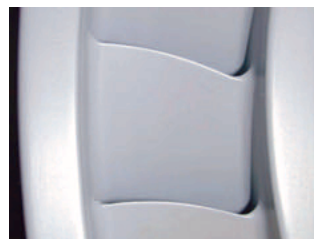
Fig. 22 Finished surface of SLA (Primer coated)
