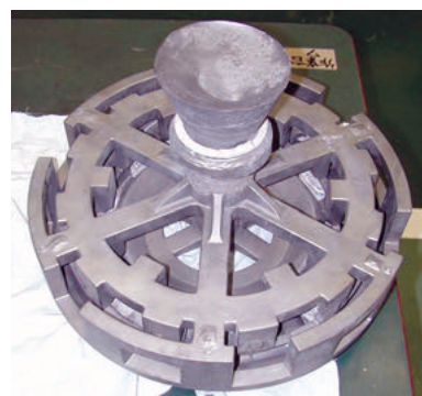
Fig. 8 As cast of turbine nozzle with gating system
