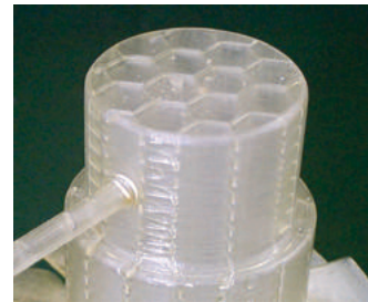
Fig. 3 Hollow model (SLA)
