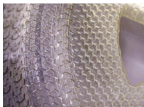
Fig. 17 Remains of support (SLA)
