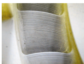
Fig. 20 Primer coated surface of SLA (Layer mark)
