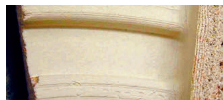
Fig. 14 No coherence (Air blowing and air vent)
