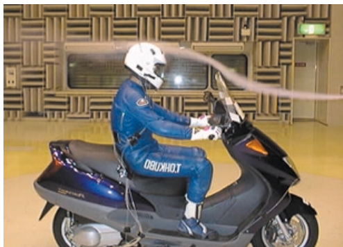
Fig. 13 Stream line of a measurement by actual scooter
