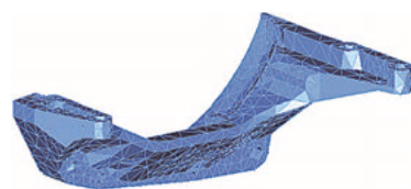
Fig. 19 FE model of gusset stiffener
