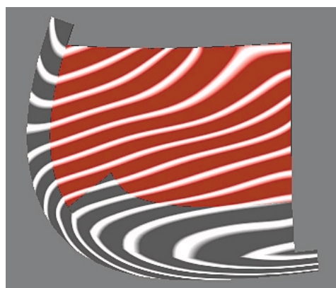
Fig. 12 Case 4: A 5-sided concave patch filled by the minimal energy method with parameters \beta=0.00001 , \gamma=0
