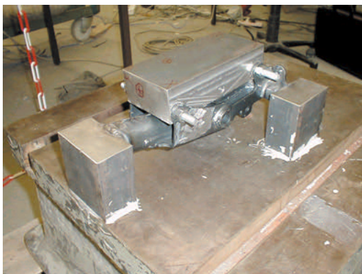
Fig. 13 Simplified model of engine frame connection and FEM model
