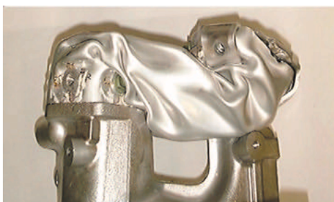
Fig. 4 Bend mode of crash frame
