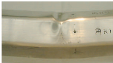
Fig. 23 Test specimen after bending test
