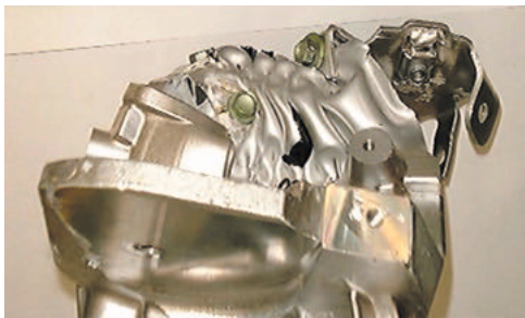
Fig. 2 Collapse mode of crash frame
