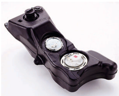
Fig. 33 External view of fuel tank
