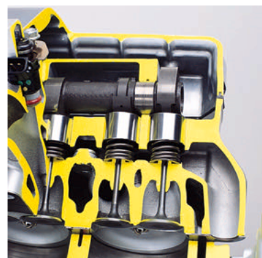
Fig. 9 Parallel two-valve train system
