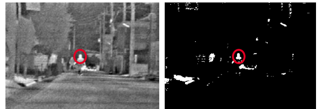
Fig.8 Infrared image and result of two level rendition in summer time condition
