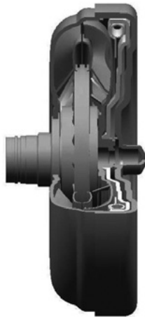
Fig.11 Side view of developed torque converter
