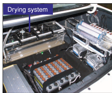
Fig.1 On-board sampling/analysis system
