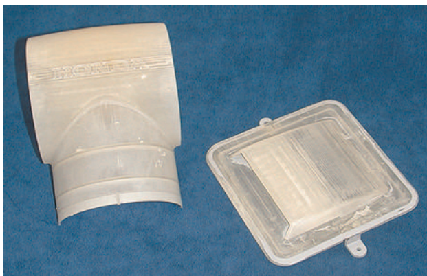
Fig.25 Rapid prototyping (SLA)
