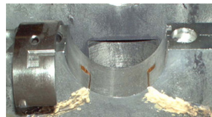
Fig.4 Strain gauge attachment
