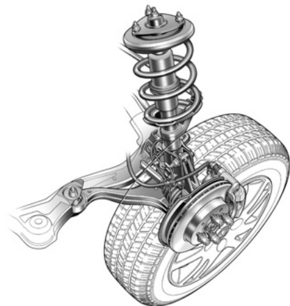
Fig. 17 Front toe control link McPherson strut suspension
