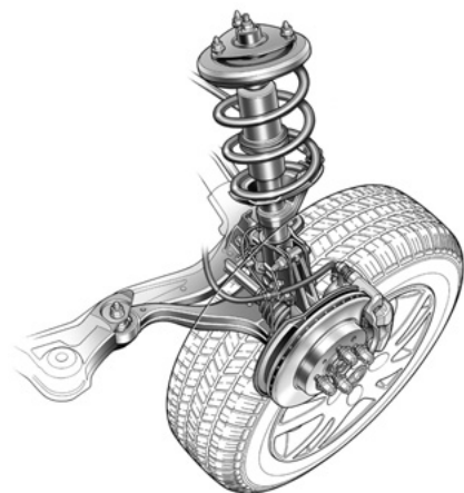
Fig. 17 Front toe control link McPherson strut suspension
