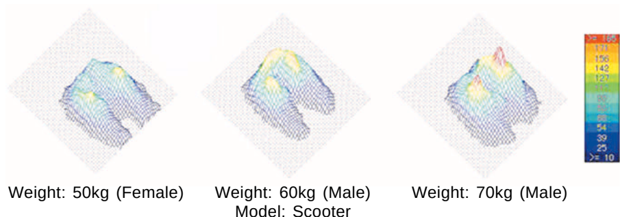
Fig.4 Body pressure distribution by rider weight difference
