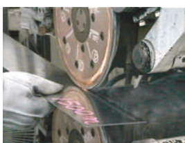
Fig.26 Seam welding test
