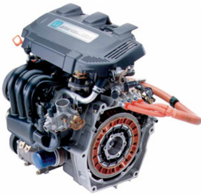
Fig.1 IMA power unit
