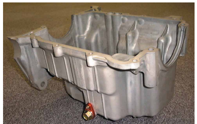
Fig.15 Appearance of magnesium oilpan using ACM522 alloy
