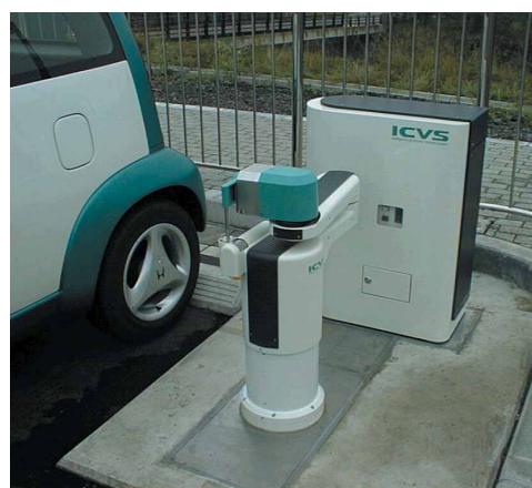
Fig.1 Inductive charger and automatic connecting unit
