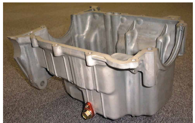
Fig.15 Appearance of magnesium oilpan using ACM522 alloy
