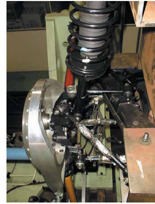
Fig.9 Suspension and rig
