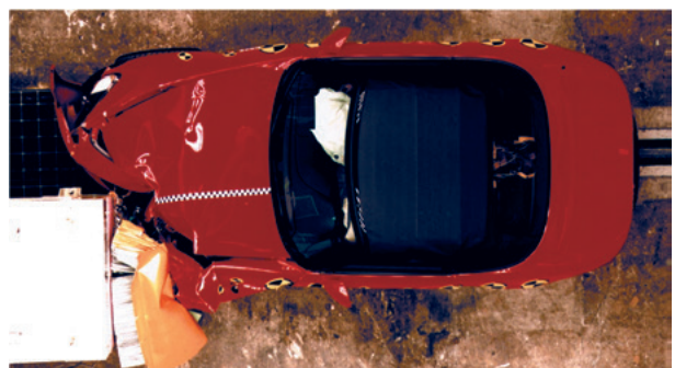
Fig.24 ODB 64km/h test result in HONDA
