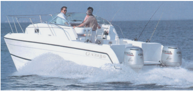
Fig.12 Cruising by a set of counter-rotated BF130s
