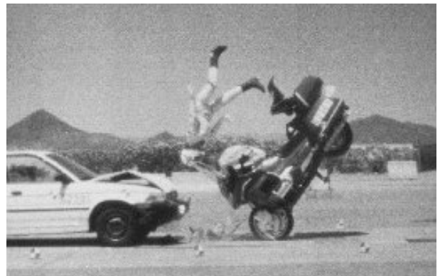
Fig.16 45mph impact test to stationary car (115-0/45)
