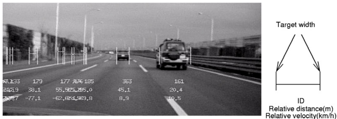
Fig.14 Real image and estimated width, distance and velocity of targets
