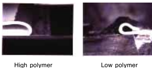
Fig.13 Effect of primer films on pulling test
