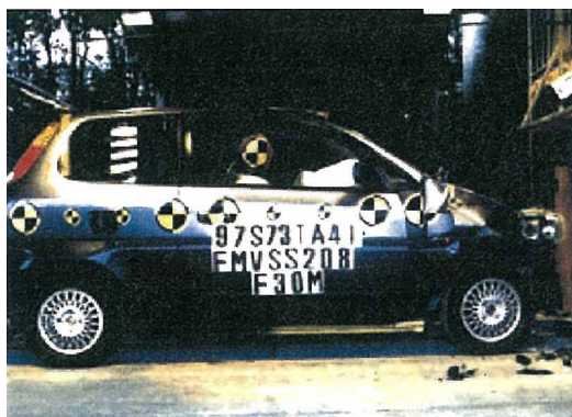
Fig.11 Head-on collision test (Fixed barrier)
